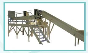
This type of a sorting plant is designed for plants with small amount of waste. The technology of sorting is similar to the small sorting plants only with the difference that the chutes by the "reading" conveyer fill movable boxes or containers, which are by a dumper emptied to a hopper of a two-chambers baler. The hopper is constructed to enable to fill both press chambers in turns from one dumping place.
