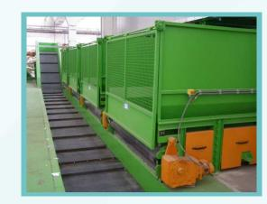
The separated waste is then transported by a system of chain conveyers with rubber belt to a chamber of the high density horizontal press, which component part is an automatic binding system for fixing the pressed bales. These are then stored by the staff on determined place before their further processing.
