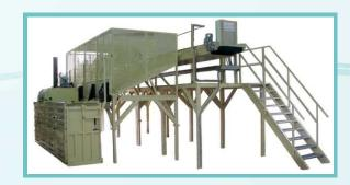
The simple sorting line has input conveyer, which transports the waste to the "reading" conveyer, where staff of three to six people sorts it and puts it to the containers, which lead directly to pressing chambers of a baler with mobile pressing head. The unsorted (residual) waste falls at the end of the "reading" conveyer to the prepared container above which there can be alternatively placed a shredder, which reduces volume of the waste for its better transport and storing.
